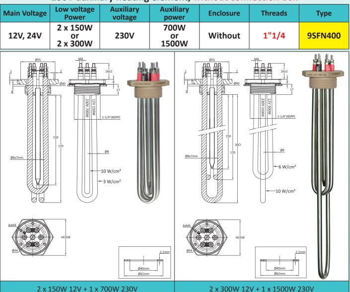
**Main application:** direct use of low voltage electricity produced by wind turbines or photovoltaic solar panels, for heating liquids, domestic hot water circuits, hot water tanks. These immersion heaters make it possible to use the surplus energy produced, and not used by domestic lighting needs or small electrical appliances. They can also be used in addition to domestic hot water tanks, limiting the need for electricity from the distribution network.
